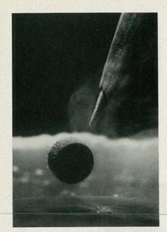
FIG. 1—A SUPERCONDUCTOR FLOATS IN air above a magnet. This experiment, which has come to symbolize the breakthroughs in superconductivity, demonstrates Meissner's effect, whereby magnetic flux does not enter a superconductive material. In effect, the superconductor looks like a "magnetic mirror."
